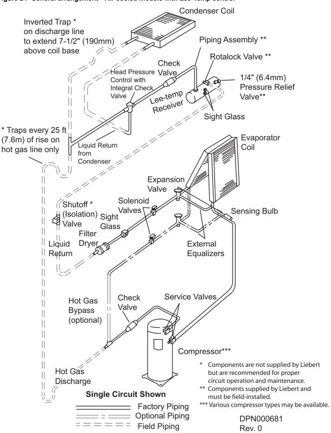
Figure 24 General arrangement—Air cooled models with Lee-Temp control
